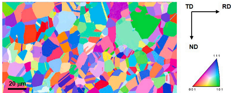
Fig. 1. The EBSD transverse direction (TD) inverse pole figure (IPF) map of the annealed material, showing a fully-recrystallized microstructure with an average grain size of 11.6 \mu\text{m} and random grain orientation.
