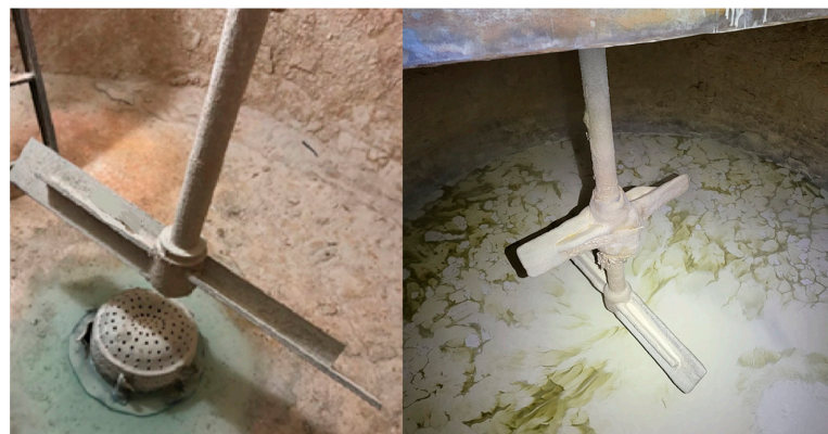
Figure 15. Single- (1440 mm) and double-stage blade installation in precipitation tank.
