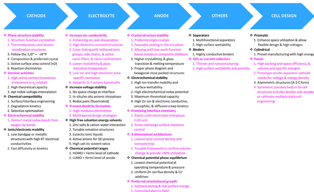
Figure 4. Illustration of key structural parameters for design of cathodes, electrolytes, anodes, separators, binders, and cell manufacturing for solid-state ZABs.
