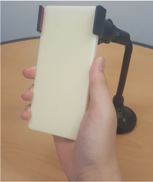
Figure 2. Smartphone mock-up mounted on a holder used in Stages 1 and 2 to minimize the effect of mass on grip comfort. (Holder clip could be moved freely to adjust mock-up angle, and the bottom was attached to the desk via suction.)
