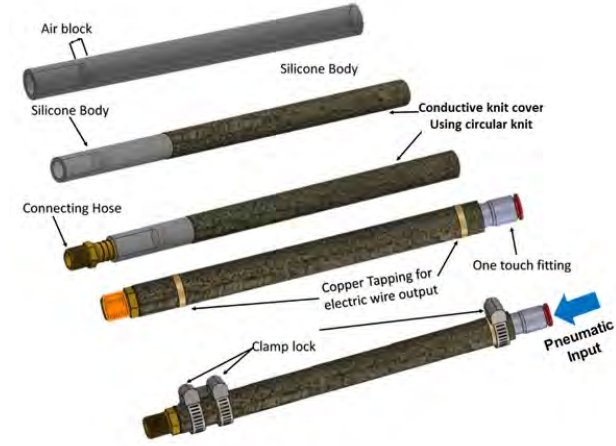
FIGURE 4. Fabrication and assembling processes of type A k-PAM actuator.
