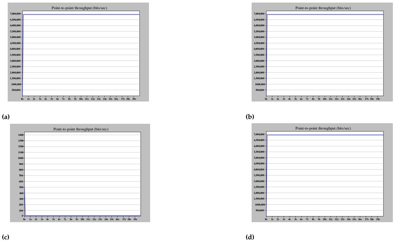
Figure 13. Attached HSR ring QuadBox links throughput simulation results. (a) Throughput of QuadBox_AB2->QuadBox_AB1 in Ring A. (b) Throughput of QuadBox_AB1->QuadBox_AB2 in Ring B. (c) Throughput of QuadBox_AB1->QuadBox_AB2 in Ring A. (d) Throughput of QuadBox_AB2->QuadBox_AB1 in Ring B.
