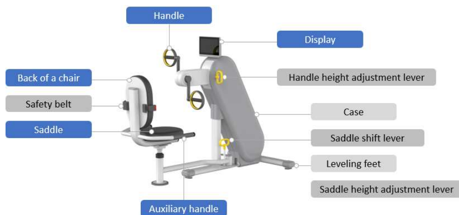
Figure 16. Second design concept of the arm ergometer applying UD.
