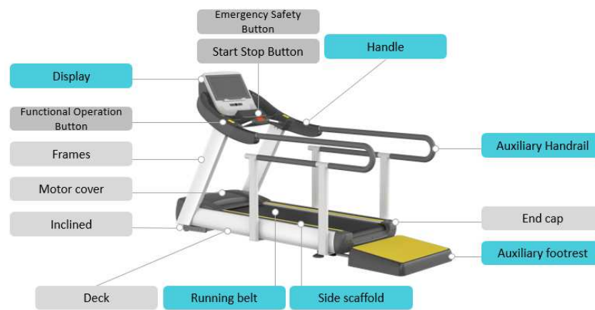
Figure 15. Second design concept of treadmill applying UD.
