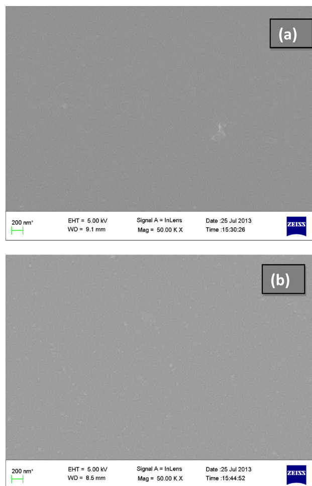
Fig. 5 FESEM images of NiO thin film deposited with a 100 W and b 200 W rf power
