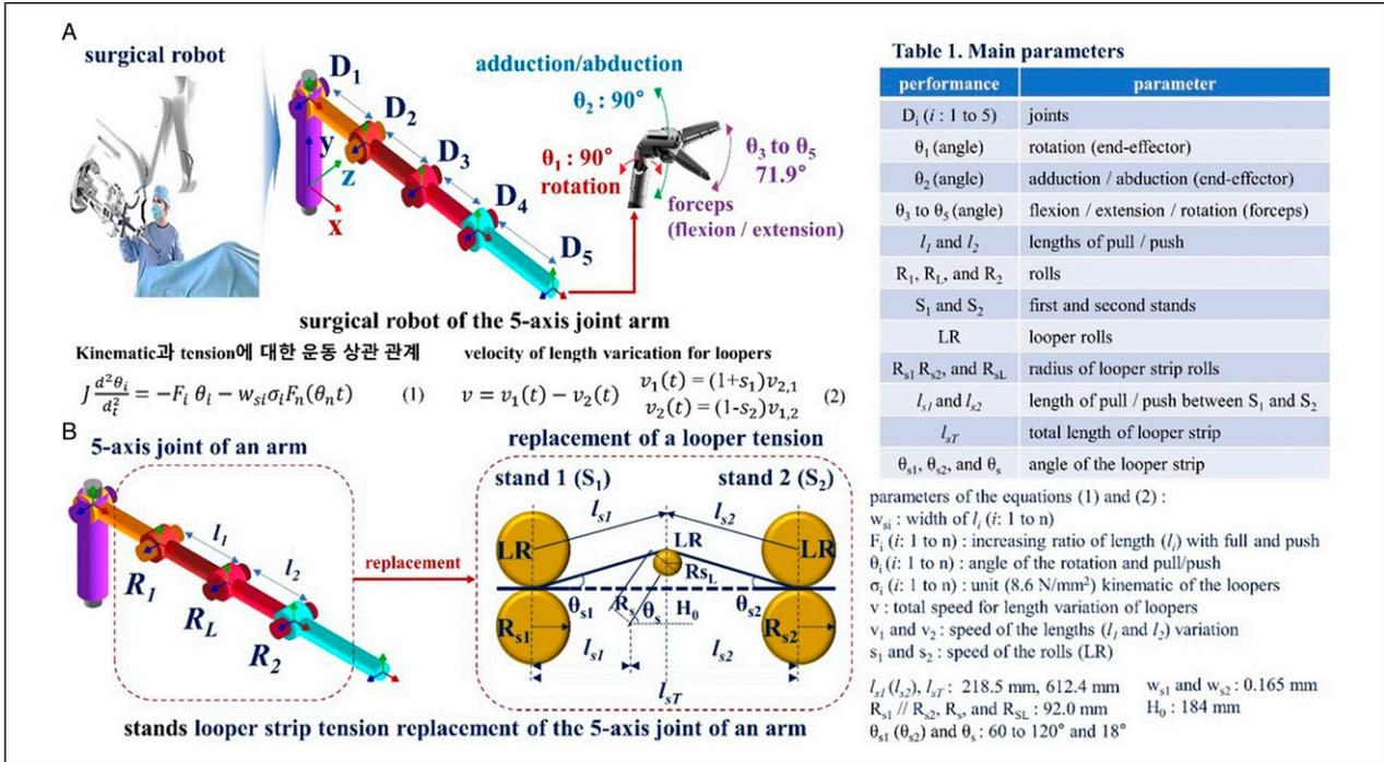
**Figure 1.** Design process of the stand and looper tension technique in the surgical robot.
