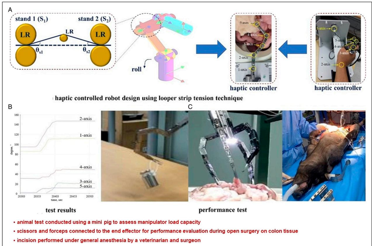
Figure 3. Performance test of the surgical robot with looper strip tension technique.
