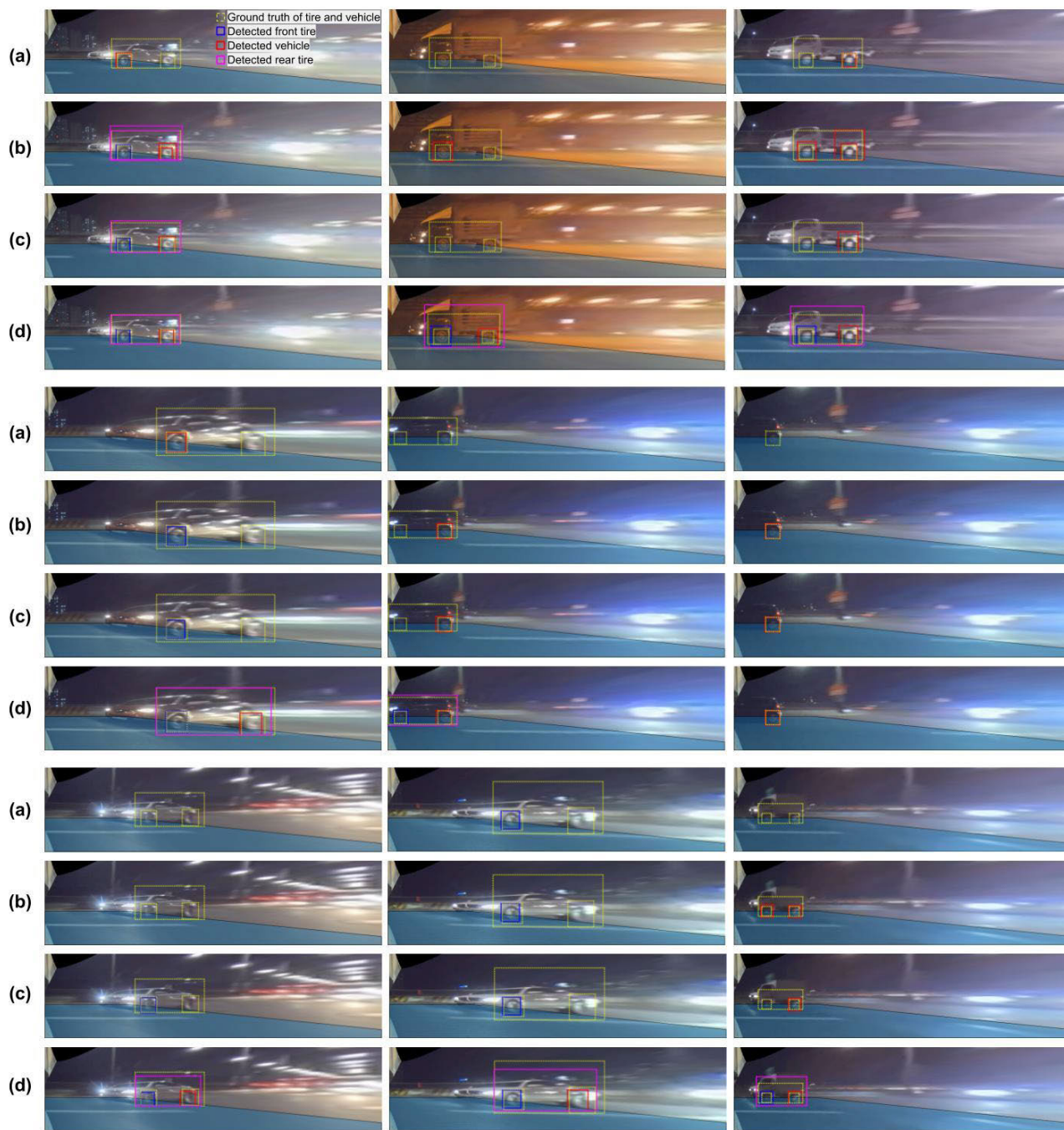
FIGURE 8. Results of vehicle detection. Training with (a) daytime samples only, (b) 500 image pairs, (c) selected 500 pairs, and (d) 2,000 image pairs.
