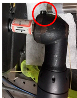
Figure 7. Vibration measurement with the accelerometer attached to the head of the nutrunner (red circle).
