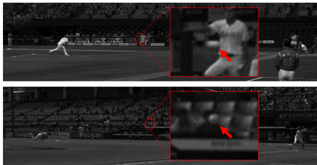
FIGURE 1. Baseball image captured during an actual game. The image resolution is 2048 \times 512 and the baseball radius is about 3 pixels.
