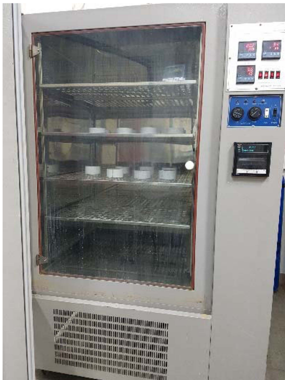
Fig. 2. Accelerated carbonation test setup.
