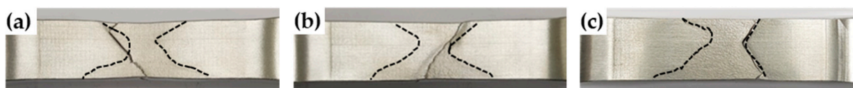
Figure 7. Fracture appearance of aluminum 5083 alloy gas metal arc welds using filler wires with different magnesium and manganese contents: (a) W1; (b) W2; (c) W3.
