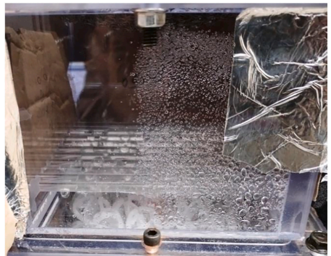
Fig. 6. Photograph of humidified air condensation across the surface of the humidifier exit with \dot{m}_a of 1 kg/min.
