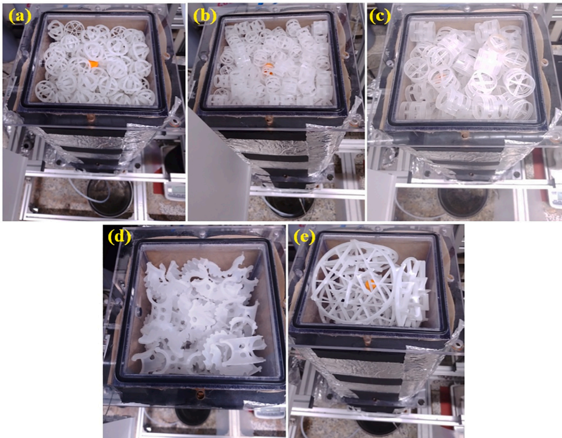
Fig. 3. Humidifier unit loaded with random packing of (a) tri-pack rings, (b) small pall rings, (c) large pall rings, (d) super intalox saddle rings, and (e) snow-flake rings.
