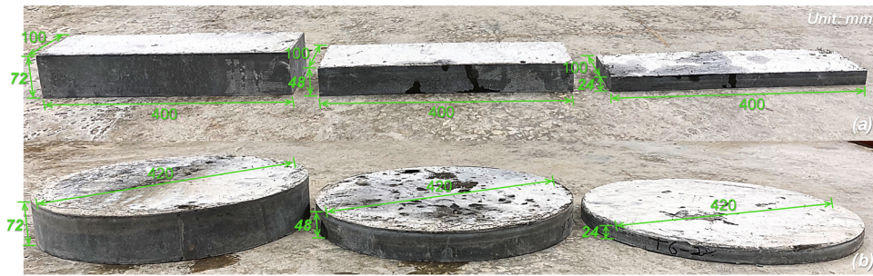
Fig. 2. Pictures of (a) uniaxial beams and (b) biaxial panels with various thicknesses of 24, 48, and 72 mm.
