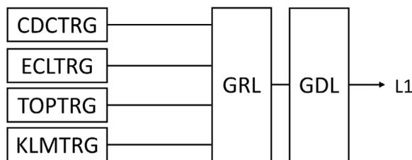
**Fig. 1.** A schematic overview of the Belle II trigger system [6]. The trigger system consists of the CDC/ECL/TOP and KLM triggers. The GRL collects all signals from each sub-trigger and delivers its matching information output to the GDL. The GDL generates a final decision with the matching information and sub-trigger outputs. L1 is the final level 1 trigger decision.
