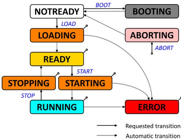
**Fig. 2.** Run control state diagram [13]. This diagram shows how the Belle II experiment handles a run. The round boxes denote the status of an NSM2 node, and the texts outside of the boxes are requests. A node status can be checked and changed by operators. The ABORTING state is reached from LOADING/READY/STOPPING/STARTING/RUNNING/ERROR states by an ABORT request (Lines with small circles connect the states to the ABORT request line).
