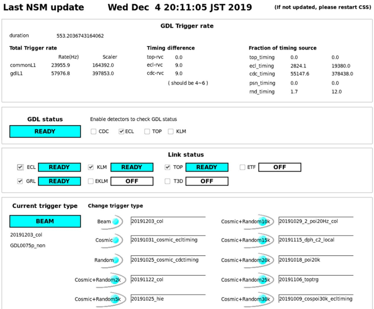
Fig. 9. The GDL detail main panel. The first block shows several real-time trigger rates. The following two blocks are for checking the GDL status. Sub-trigger status and link status can be included/excluded to generate the GDL status with checkboxes. The last block is for setting the trigger type. Trigger type and related parameters can be changed with the ellipse-shaped button.
