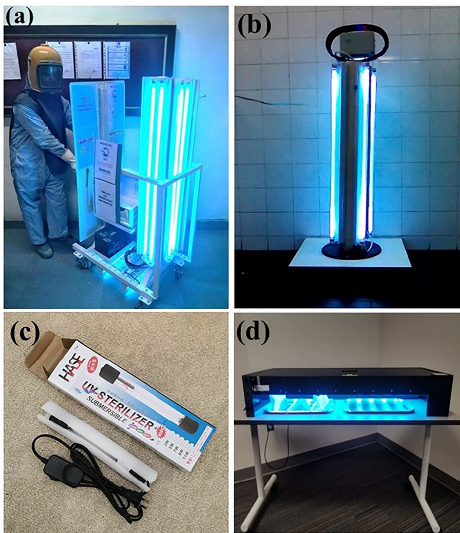
Fig. 4. Pictures of several germicidal devices that are based on UVC radiation for deployment in indoor places and respiratory masks (a) A UVC-disinfection based trolley prototype developed by Mekins Industries, Hyderabad, India for the rapid disinfection of hospitals (b) UV-C device working developed for disinfection of rooms (Bentancor and Vidal, 2018) (c) A portable UVC disinfection lamp developed for daily sterilization of essential items, toys, electronics and small areas. (d) UV device developed by Daavlin International for decontaminating respirators and other essential items (Hamzavi et al., 2020).
