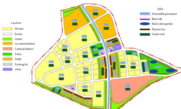
Figure 6. Overview of the deployment of LID techniques.
