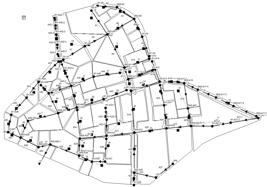
Figure 5. Layout of the drainage system.
