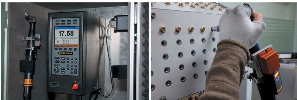
Figure 2. Electric fastening tool system (left) that, when it pushed on the panel, automatically fastens the bolt and collects real-time torque values (right).
