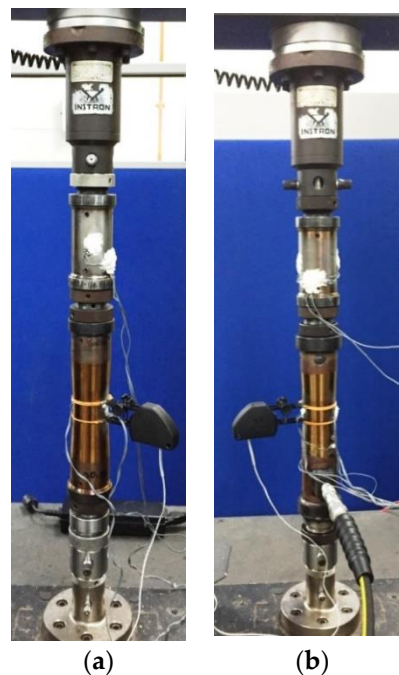
Figure 5. Experimental setup of specimens: (a) Uniaxial (b) Biaxial.
