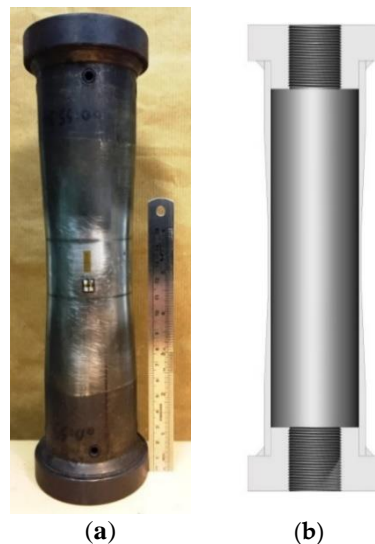
Figure 2. Monotonic uniaxial test sample: (a) external view (b) internal view.
