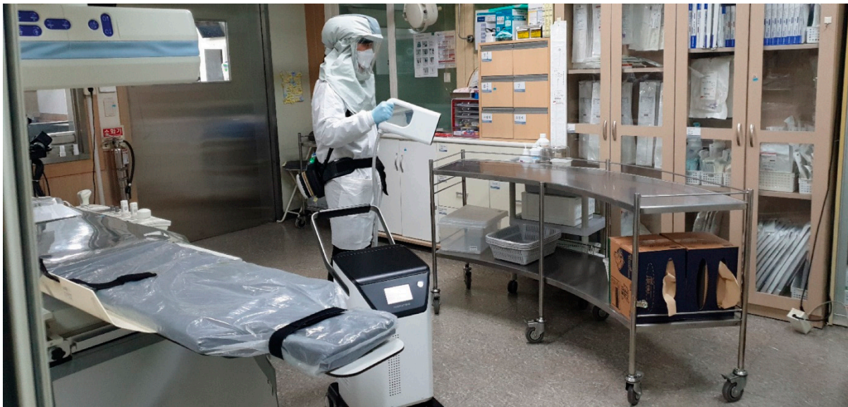
Figure 1. Plasma-treated hydrogen peroxide mist disinfection in a hospital environment using a PlaClin ® disinfectant and disinfectant containing 5.9% w/w hydrogen peroxide.
