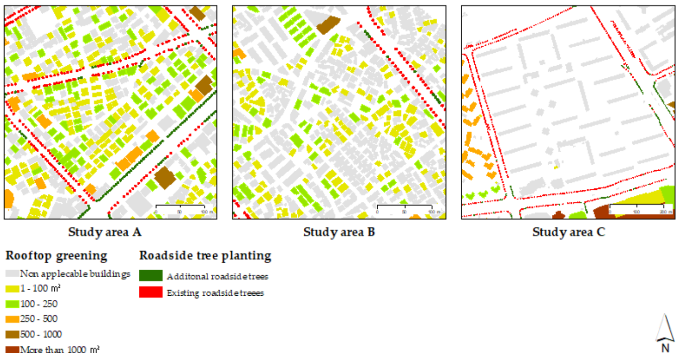
Figure 8. Analysis results of locations suitable for roadside tree planting in case study areas A, B and C.
