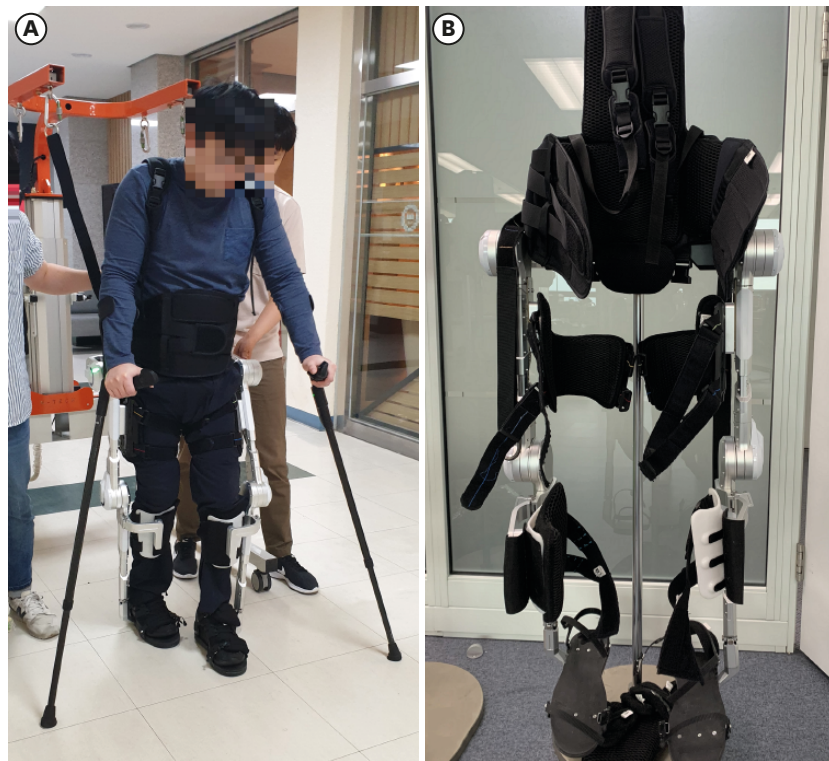
Fig. 1. The H-MEX wearable powered exoskeleton (A) worn by the participant and (B) after takeoff. H-MEX = Hyundai Medical Exoskeleton. The figures are published under agreement of the patient.
