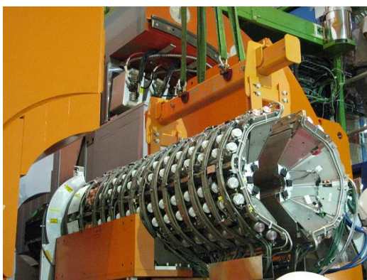
Figure 2. Left: closeup image of the CASTOR calorimeter surrounded by the CMS collar shielding in the open position during an integration test, about 5 m below the beam pipe. Right: visualization of the CASTOR detector integrated around the beam pipe. The CMS interaction point is at 14.4 m upstream (towards the upper right). The TOTEM T2 tracking station, and several pieces of LHC/CMS infrastructure, are visible along this direction.
