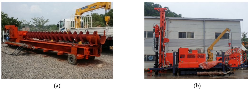
Figure 2. Comparison of boring machine: (a) outdated boring machine, and (b) newly developed high-performance MSP boring machine.
