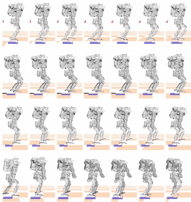
FIGURE 6. The simulated results of the standard , no-action-range , SIMBICON-stancehip , and fixed-duration policies (top to bottom). The images are captured at 0.133 second time intervals for each column.
