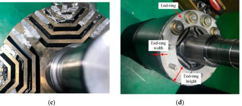
Figure 14. Manufactured LS-SynRM (a) rotor core, (b) endplate for die-casting, (c) cross-section of rotor, (**d**) rotor with the end-ring.
