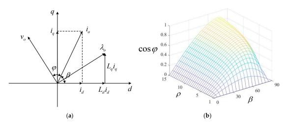
Figure 3. Characteristic of LS-SynRM (a) vector diagram, and (b) power factor.
