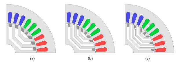
Figure 6. FEA model according to the number of barriers (a) model 1, (b) model 2, and (c) model 3.
