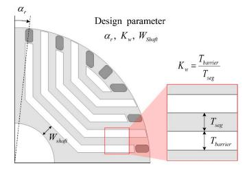
Figure 7. Design parameters for the optimal design using the response surface method (RSM).
