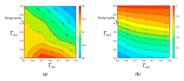
Figure 12. FEA result according to the design parameter of rib (a) safety factor, and (b) power factor.
