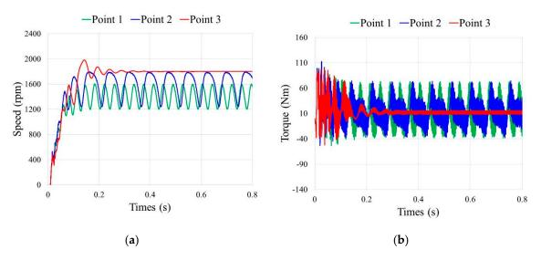
Figure 10. Speed and torque curve of the selected three points (a) speed curve (b) torque curve.
