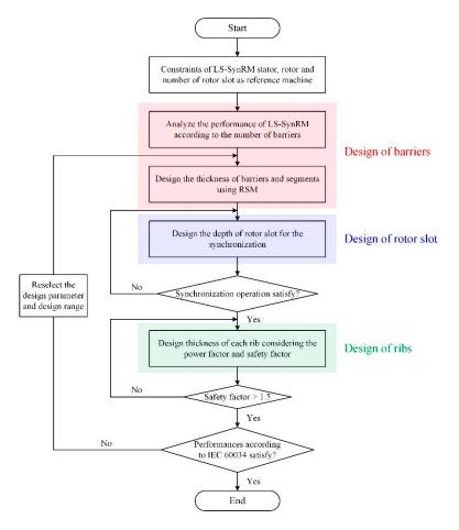
Figure 5. Design process of LS-SynRM.
