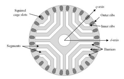
Figure 1. Rotor structure of the line-start synchronous reluctance motor (LS-SynRM).
