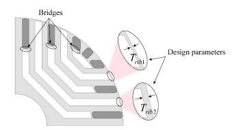
Figure 11. Design parameter for the power factor and safety factor.
