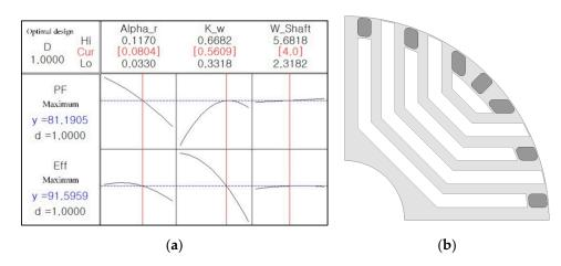
Figure 8. Optimization using RSM under rated current condition. (a) RSM result, (b) optimal design result.
