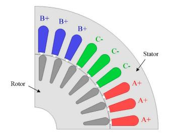
Figure 4. Finite element analysis (FEA) model of reference machine.
