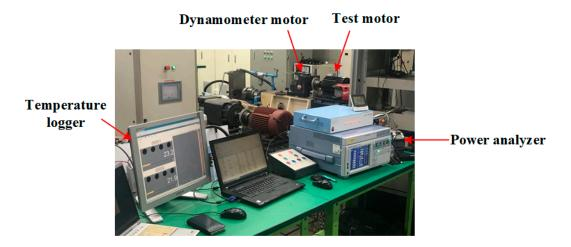
Figure 15. The experiment environment and test dynamometer.
