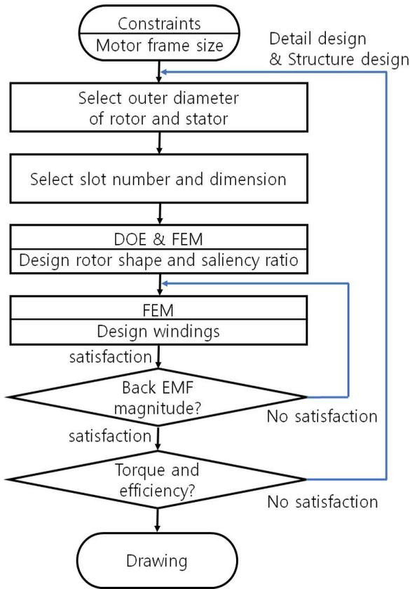
Fig. 5. SynRM rotor design algorithm using FEA
