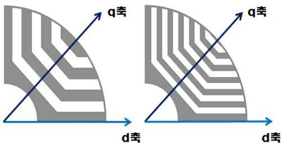
Fig. 2. Rotor shape according to barrier number
