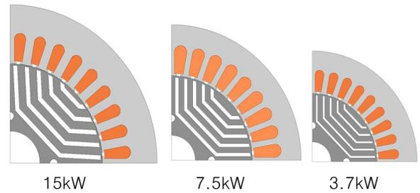
Fig. 6. Designed rotor for each output power
