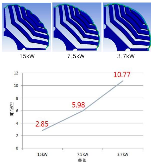
Fig. 7. Stiffness analysis for each output power
