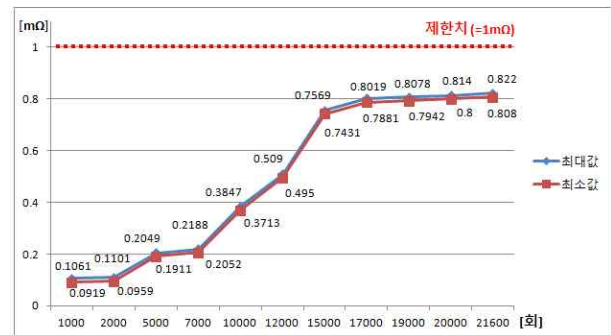
Fig. 3. DC(+) Contact Resistance of Couplers considered with Measurement Uncertainty
