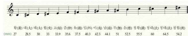
Figure 3. The 16 notes of the modern pyeongyeong , the Korean (and Chinese character) names of each pitch and the average thickness of each chime (in mm).
