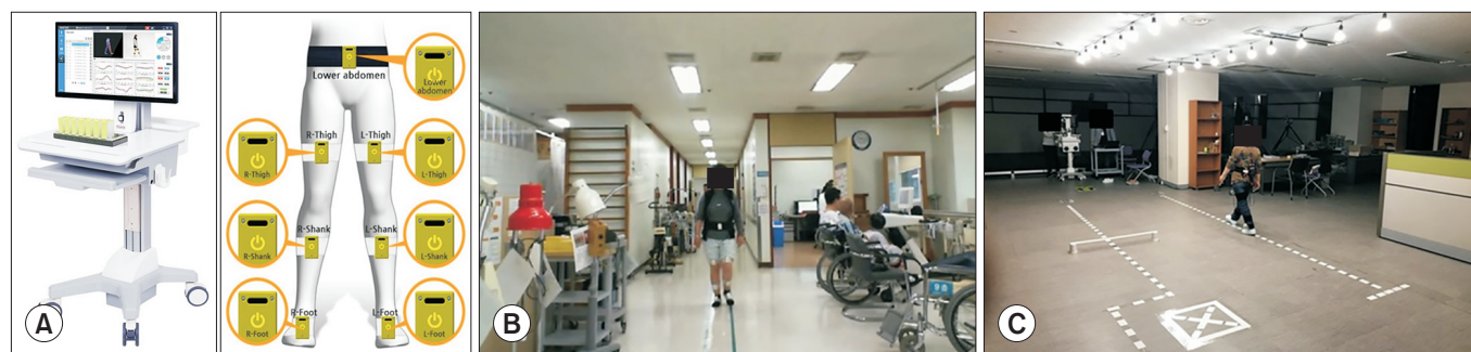
Fig. 1. A hardware of the gait analysis system consisting of PC and wireless IMU sensors (A), and gait trial of knee osteoarthritis patient (B) and normal subject (C). IMU, inertial measurement unit.
