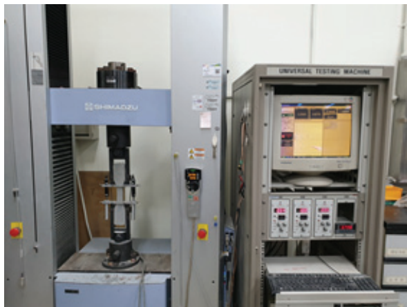
Fig. 3. Universal Testing Machine (300 kN)
