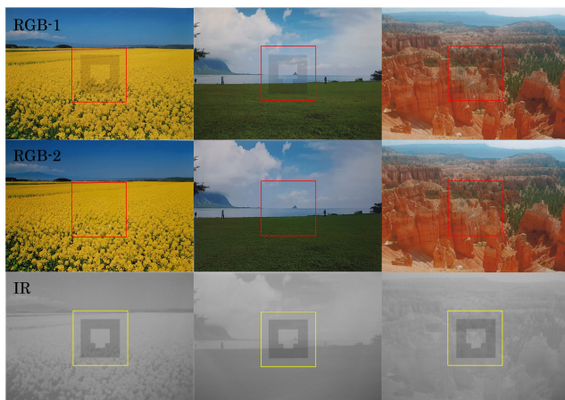
FIGURE 13. Metamer marker applied to the photo. (RGB-1) Overlaid printing of photos and marker, (RGB-2) Overlaid printing of color-corrected photos and marker, (IR) Infrared camera image (RGB Captured by mobile phone S10+).
