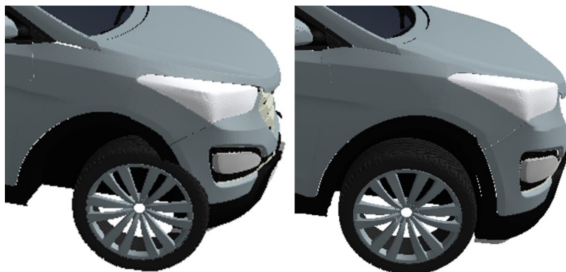
Figure 11. Comparison between deformed bumper without translated wheels (left) and with translated wheels (right).
