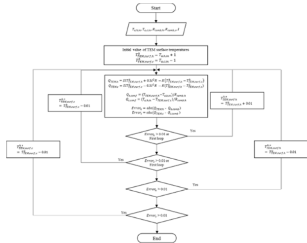
Figure 5: Simulation logic of the thermoelectric module.
