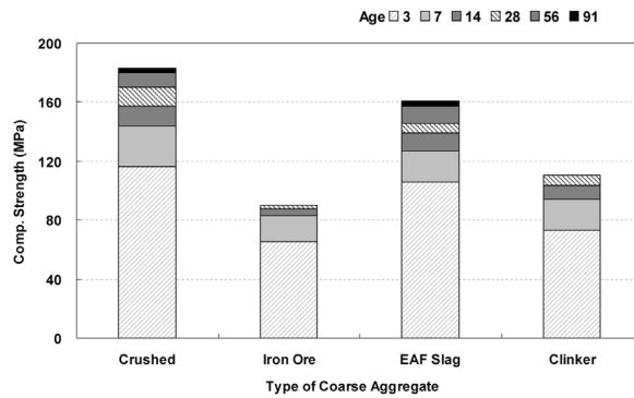
Fig. 14 – Effect of coarse aggregate type on the compressive strength (Note: Compressive strength of concrete with iron ore and clinker was only measured until 28 days).
