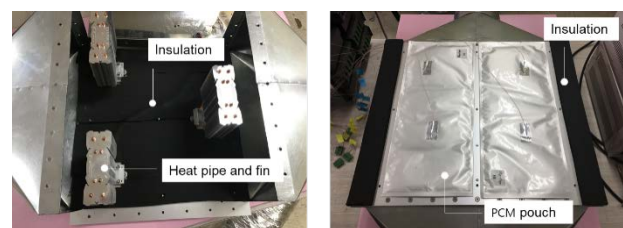
Fig. 4. Interior part of the PCM–TERCP mock-up model.
