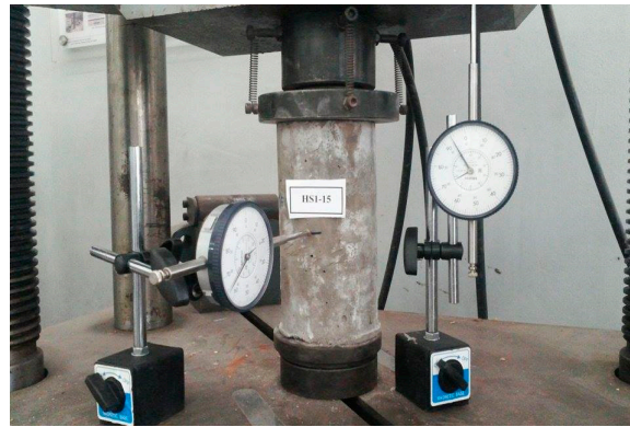
Figure 7. Experiment of Poisson's ratio and elastic modulus.
