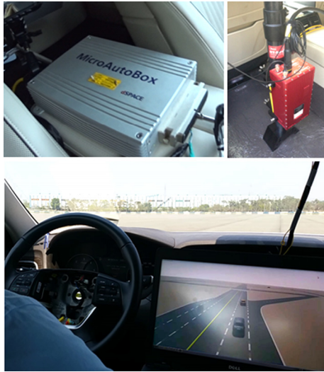
Photo. 1 VIL equipments RCP, GPS/INS and testing scene
