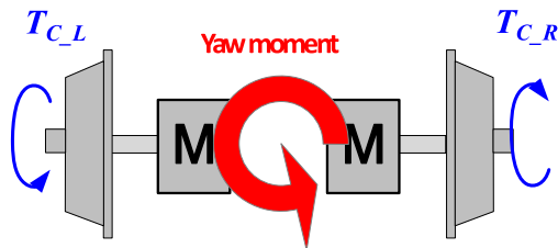
FIGURE 3. Generation of yaw moment through independent torque control.
