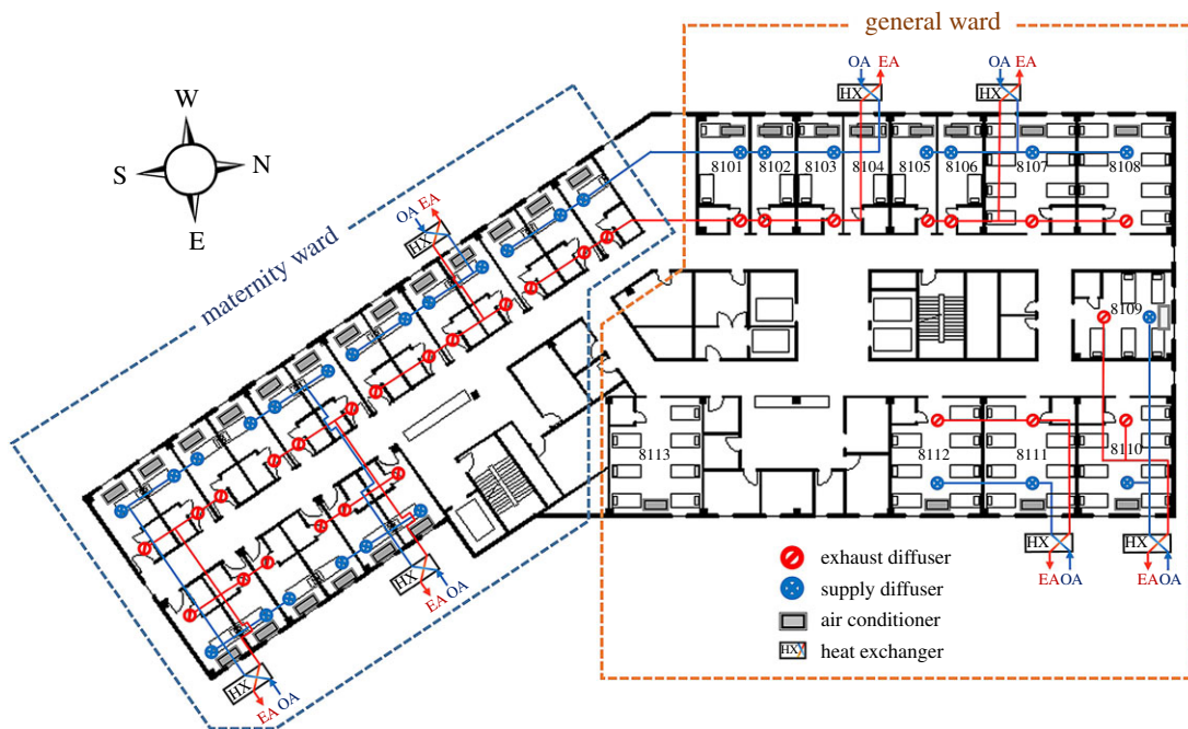
Figure 1. Layout and mechanical ventilation system of Pyeongtaek St Mary's hospital 8th floor.
