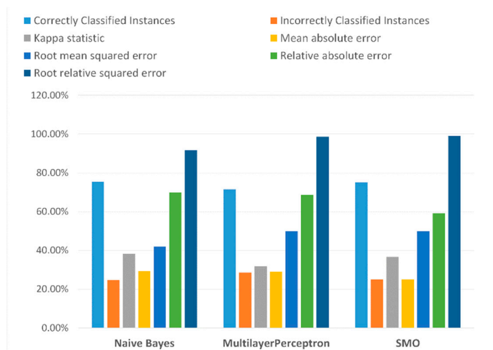
Figure 12. Workload analysis algorithms: Naïve Bayes, multilayer perceptron, and SMO comparisons based on correctly classified instances, incorrectly classified instances, Kappa statistic, mean absolute error, root mean squared error, relative absolute error, and root relative squared error.
