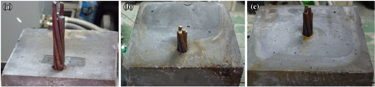
Fig. 5 Pictures for pullout test specimens after complete testing; a c = 1d_b , b c = 2d_b , and c c = \text{center} .
