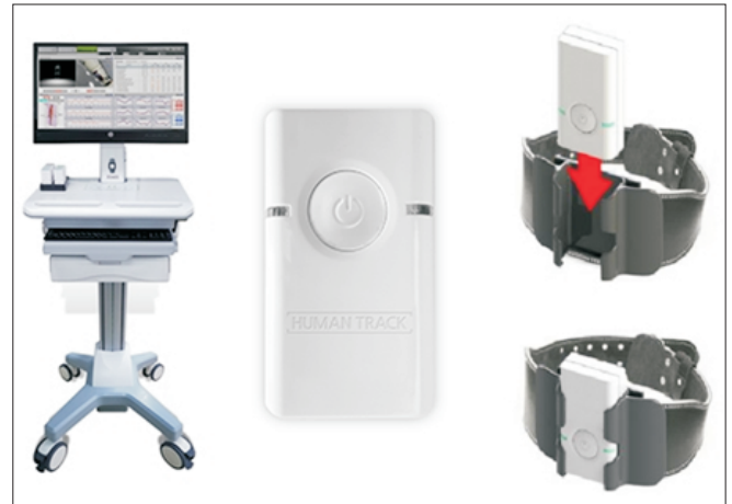
Fig. 2. The inertial measurement unit sensor is placed on a holder so as to increase stability and accuracy.
