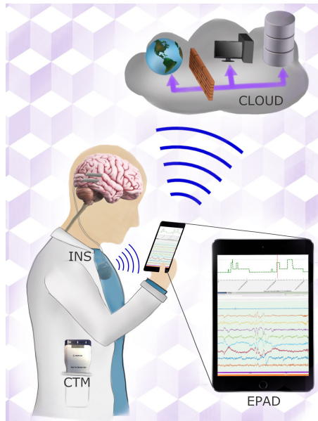
FIGURE 1. Schematic of next generation epilepsy management system using Medtronic investigational Summit RC+S. The implanted neural stimulator (INS) combines flexible stimulation paradigms, continuous telemetry of intracranial EEG, bi-directional communication between the INS and the Mayo Epilepsy Patient Assistant Device (EPAD) and provided by the Clinician Telemetry Module (CTM) and Summit RDK. The EPAD seamlessly interfaces with the INS and cloud to create a flexible platform with local and distributed computing, analytics, and data storage.
