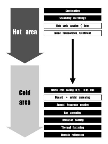
Figure 4. Maximum process shortening in the hot area by direct casting to less than 3 mm [23].
