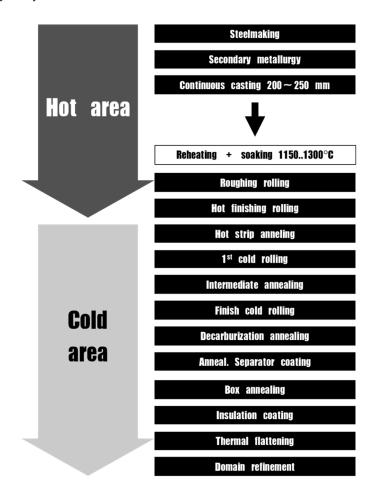
Figure 3. Production schedule with low temperature slab reheating of grain-oriented steel [23].
