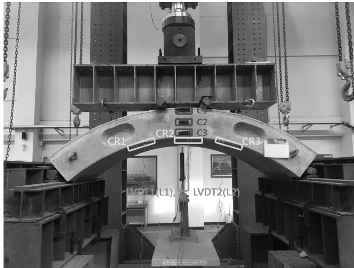
Concrete gage: C1, C2, C3 Crack gage: CR1, CR2, CR3 LVDT: L1, L2
