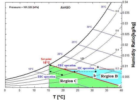
Figure 4. Process of outdoor air handling in regions B and C
