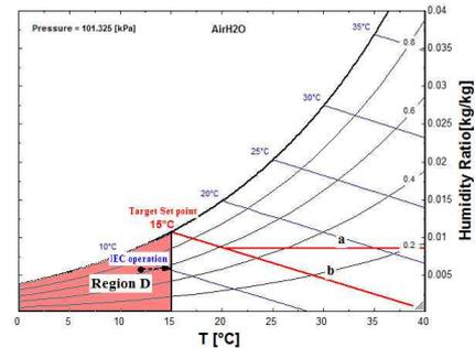
Figure 5. Process of outdoor air handling in regions D
