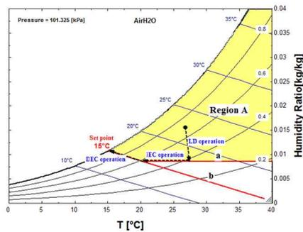
Figure 3. Process of outdoor air handling in region A
