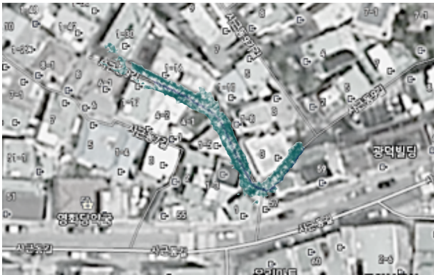
Fig. 12: An outdoor trajectory (length : 85m) on the street is overlaid on the real map. The difference between the estimated end points and the points on the map is 1.2m. The green dots represent the 3D landmarks reconstructed by the proposed algorithm.
